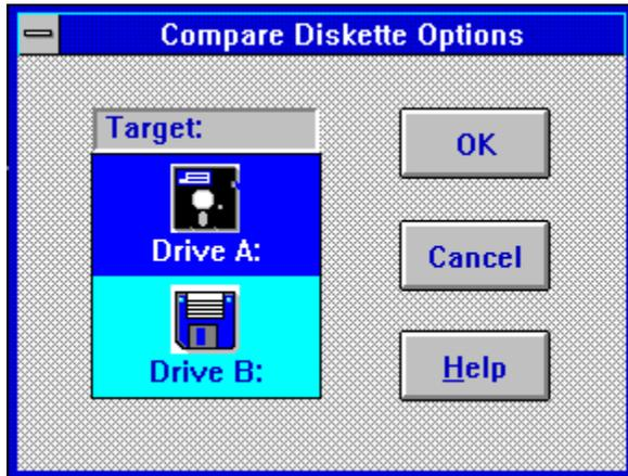
**Note:** If a device driver such as **Stacker** is enabled during the write operation, a follow-on compare operation will most likely fail, even though the file data on the target diskette matches the source diskette. This occurs because drivers such as Stacker sometimes update the target diskette during write operations. These updates are to device driver areas of the diskette and do not affect files copied to the target diskette.
