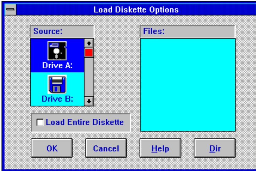
Loads a diskette image from diskette into memory. Select the Load All Tracks option if you desire to read all tracks. The default is to read only up to and including the last track containing data.
