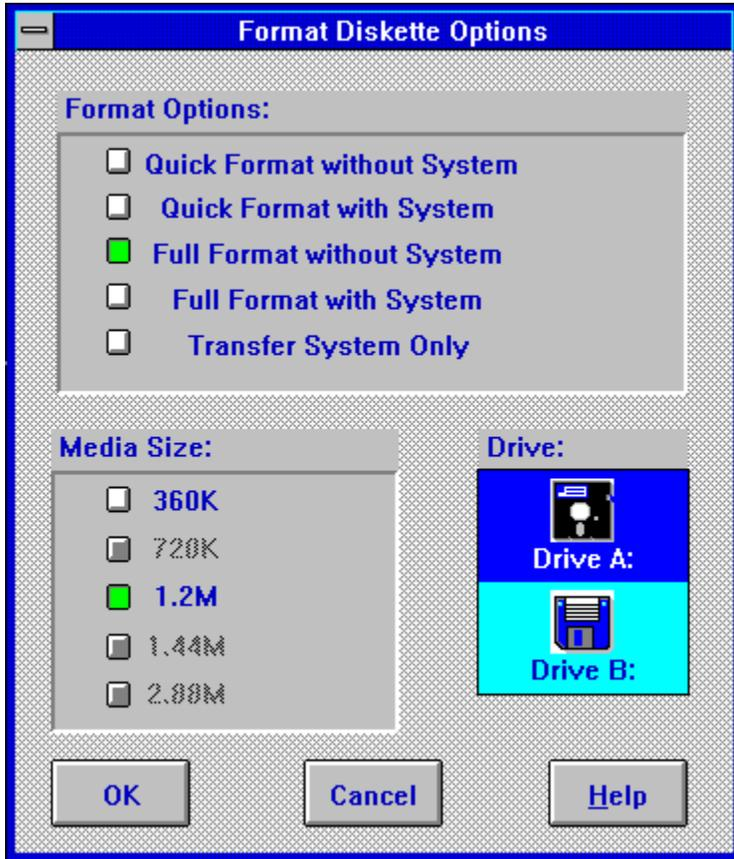
The Quick Format option simply initializes the Boot Sector, the File Allocation Tables and the Root Directory. The Quick Format will work only if the target diskette has been previously successfully formatted.
